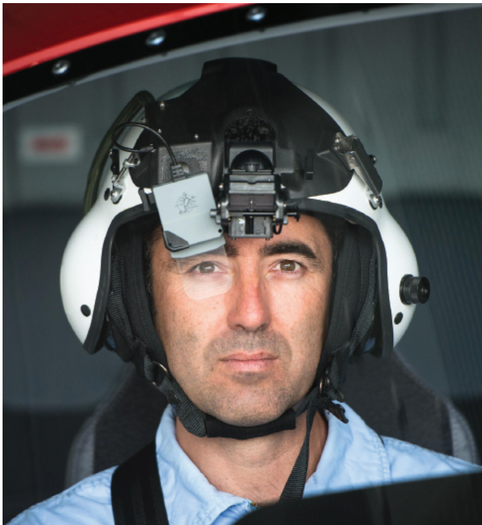
‘Eyes-out’ helmet-mounted display derives from military solutions and weighs just 400g
