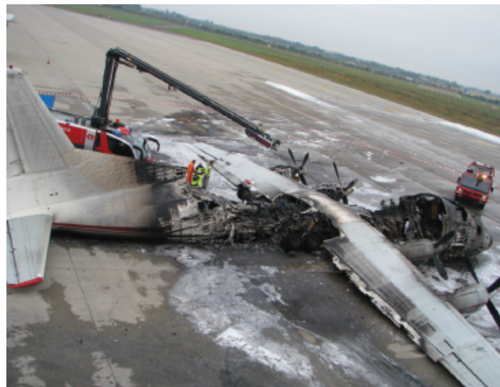
Severity of An-12 blaze was exacerbated by fuel leak from floor tanks
